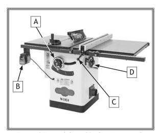
Figure 27. Model W1824 basic controls.
